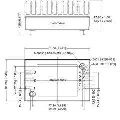
Note: Unit:mm[inch] Pin1.2.3.5.6.7's diameter: 1.00[0.039]
