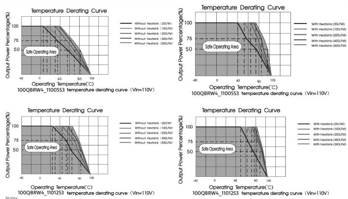
1. Temperature derating curves and efficiency curves are typical test values.
