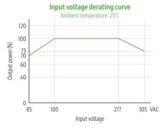
1: Input Voltage should be derated based on Input voltage derating curve when it is 85~100VAC/277~305VAC/120~140VDC/390~430VDC
