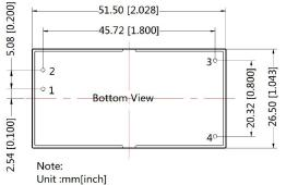
Pin diameter tolerances :±0.10[±0.004] General tolerances:±0.50[±0.020]
