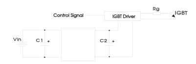
C1/C2 100uF/35V (Low internal resistance capacitance)
