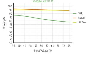
**Efficiency Vs Input Voltage**
