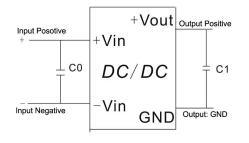
Input reflecting ripple current test circuit:
