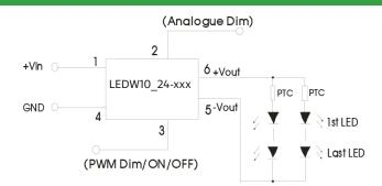
If it is necessary to protect LED in actual application, you could connect a PTC to the input of every channel or all channels, as shown in Recommended AC input circuit.
