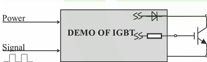
Diagram 20: Principle of GAPTEC DEMO board and its terminals
