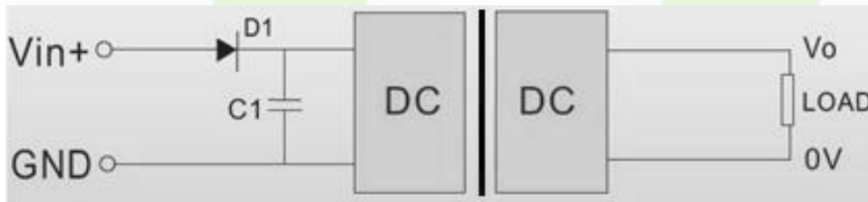
Diagram 3-6 Input reverse polarity protection circuit
